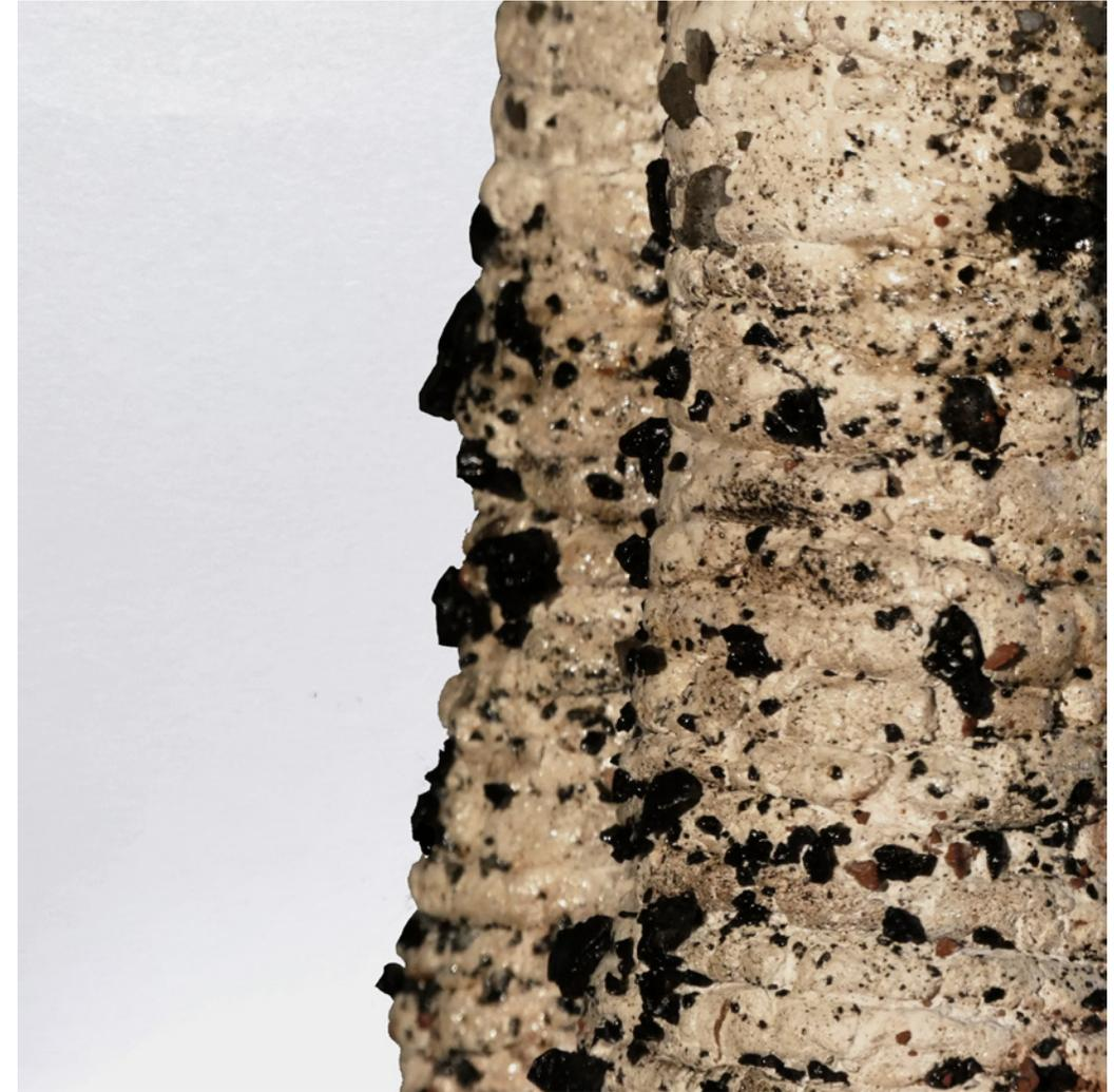
From the base to the opening, the hearth is made up of organic material from waste cleaning, bricks and asphalt from early masonry experiments, concrete from the joinery models, and wood blended from the offcuts of the timber frame.
