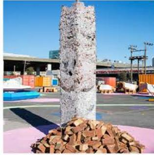
"Clastic Order is a series of free-standing columns made by combining reclaimed construction debris with post-industrial plastic waste, and the first full-scale demonstration of T+E+A+M's ongoing research on the strategies and **aesthetics of reassembly.**"
