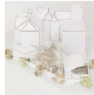
"The **construction** of the roof and deck exploit the tendency to accumulate waste that building practices typically produce. Rather than **discard material** remnants off-site, excess is cut and refit into the project for use."
