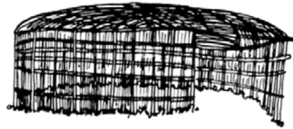
STAGE 4 placing infill branches and thatch
