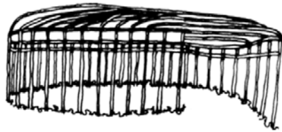
STAGE 3 constructing roof structure by criss crossing and fastening members
